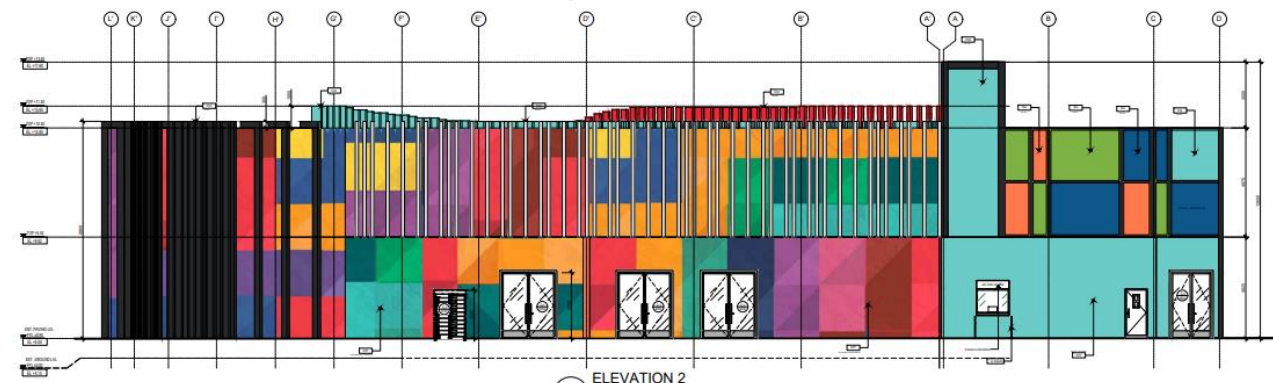
02 ELEVATION 2 ARRIVAL ZONE ENTRANCE GATE - SCALE 1:100
